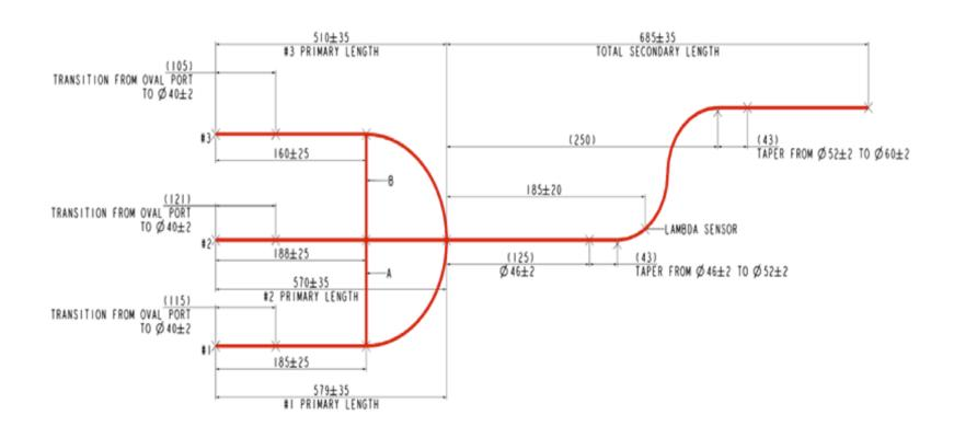
• All pipe diameters shown are internal diameters.
